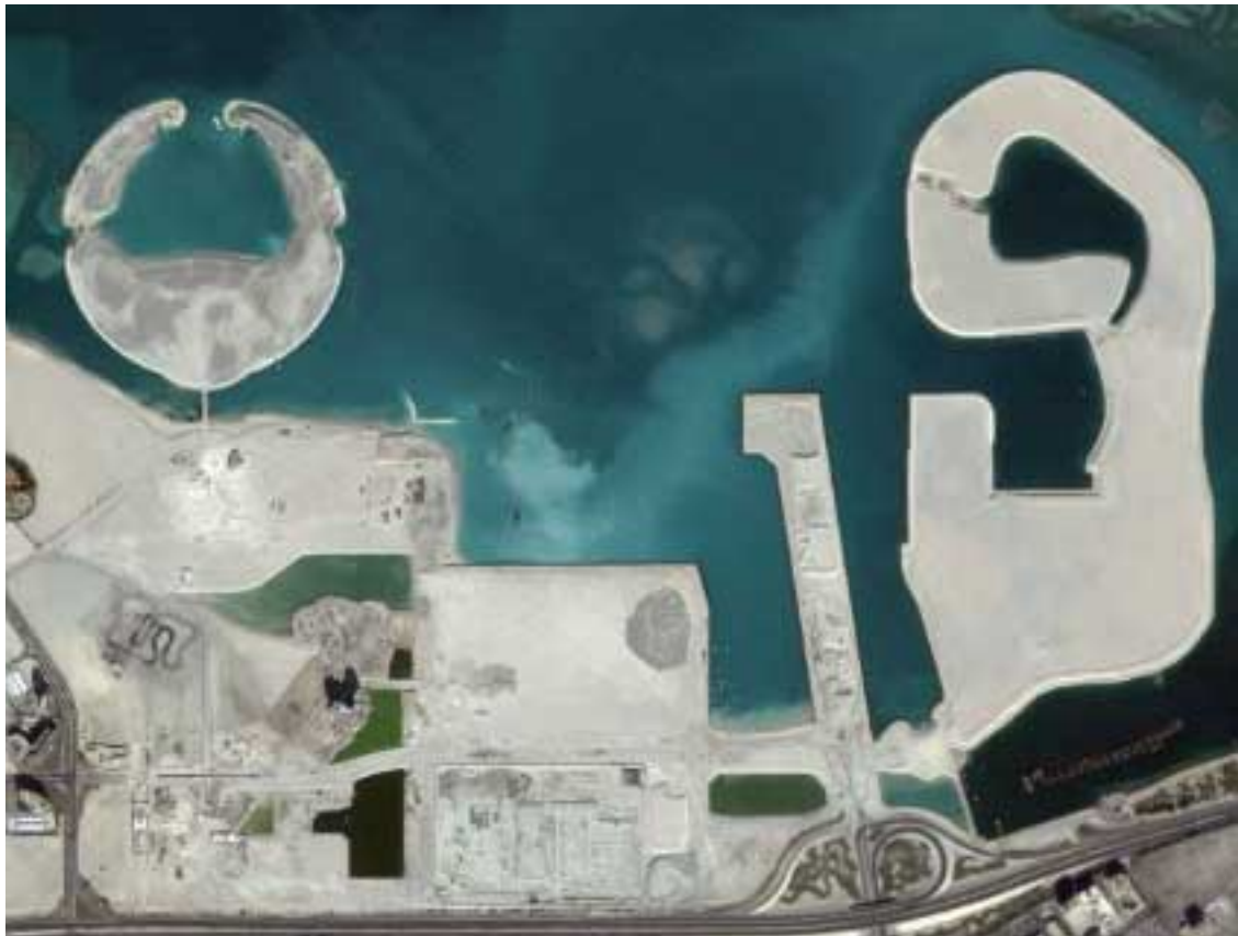
Figure 5: New development along the NW sector of Manama, showing the extensive filling operations taking place to reclaim land for Gulf-front development.
